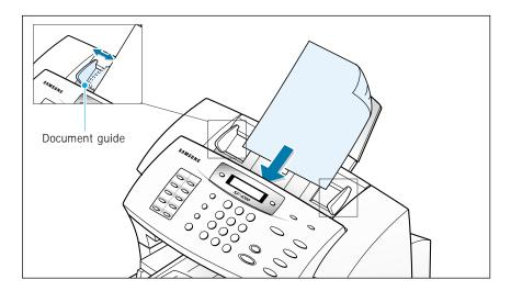
You can insert up to **30 sheets at a time**. If you insert more than one sheet, ensure the bottom sheet enters first. Stagger the leading edge of the document slightly, and insert the document with a slight push to ensure they feed smoothly.
